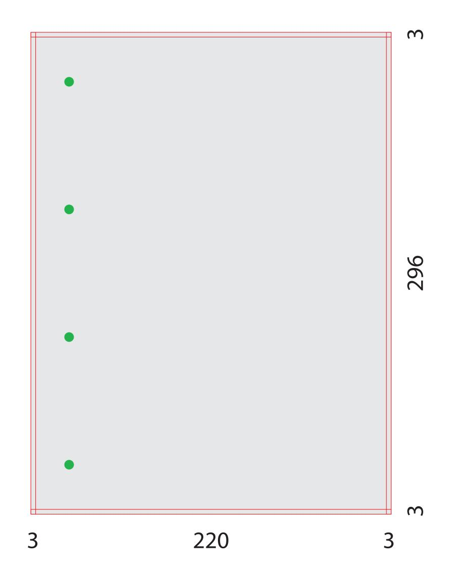
In the cover sheet, 4 holes are drilled in the final block (marked in green in the drawing - must not be part of the graphics)
